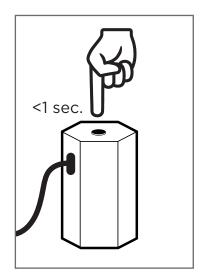
**1.** Plug the Beekee Box into a power adapter and shortly press the button.
